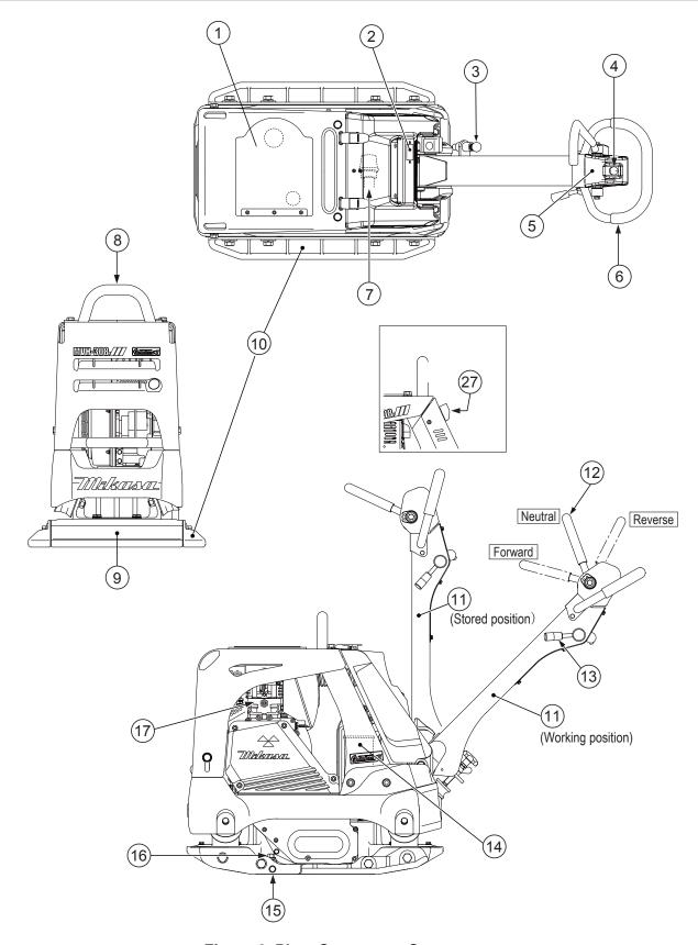
**Figure 2. Plate Compactor Components**
